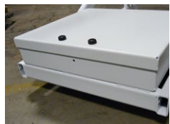
Hidden Ballast Compartment
