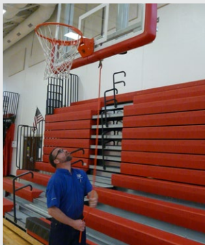
Standard Manual Crank Operation
