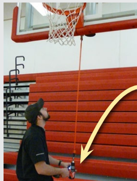
Optional BA931 Cordless Winch Winder Operation
